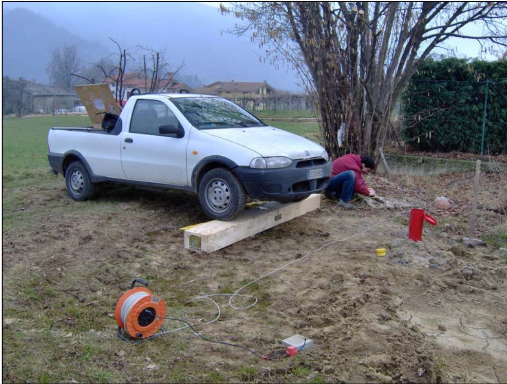
Figura 5 Prova down-hole S1
